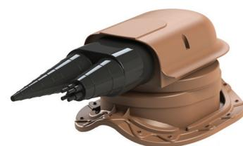
VILPE has developed and manufactured pass-throughs of the highest quality for decades. The Solar pass-throughs include a preattached coupling ring. Furthermore, the pass-through set includes a flange, a cover, a shrinking tube and the screws needed for installation. The size of the pipe hole in the front of the Solar passthrough is 100 mm x 60 mm. For  $\varnothing$  4 - 50 mm cables and wires there is also separately available Solar Cable Sealing.
