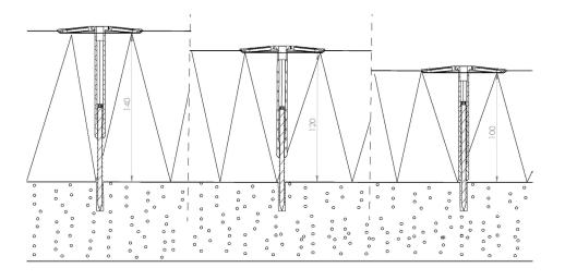
In the example image, the 100 mm fastener is adjusted to fit the insulation cover of 100, 120 and 140 mm.
