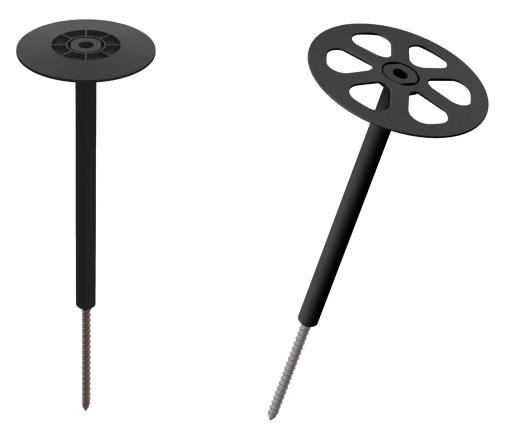
A flexible insulation fastener for easy installation. Only a 30 mm deep hole made with a 5 mm concrete drill bit is required for installation.
