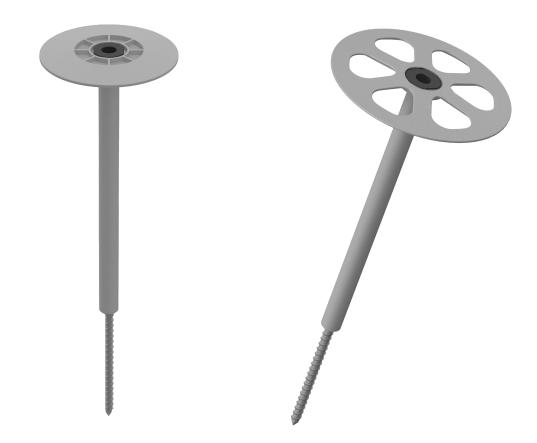
A flexible insulation fastener for easy installation. Only a 30 mm deep hole made with a 5 mm concrete drill bit is required for installation.
