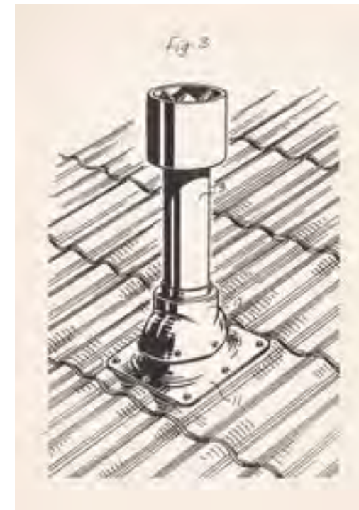
Eero’s drawing of the first VILPE sewer exhaust pipe (Ø 110 mm) from 1988. The name VILPE came into being from this product.
