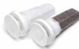
Visible pollution collected on a used filter.
