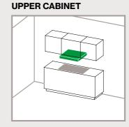
The cooker hood is installed under the upper cabinet.
