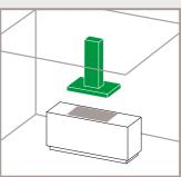
The hood is mounted on the ceiling.
